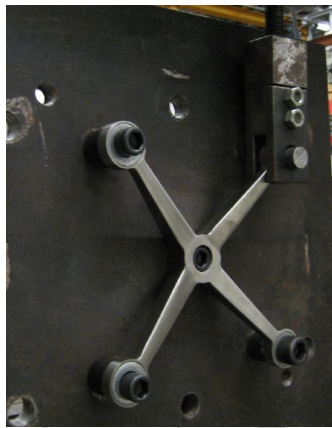
Photo. 5: Test setup-Spider fitting (CKS-F200-4)
