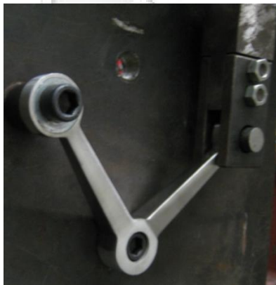
Photo. 6: Test setup-Spider fitting-CKS-F200-2
