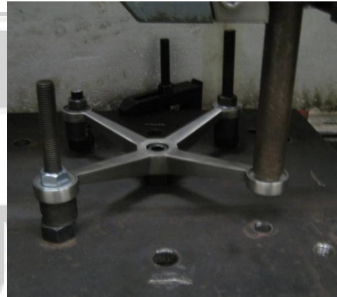
Photo. 5: Test setup-Spider fitting (CKS-F200-4)
