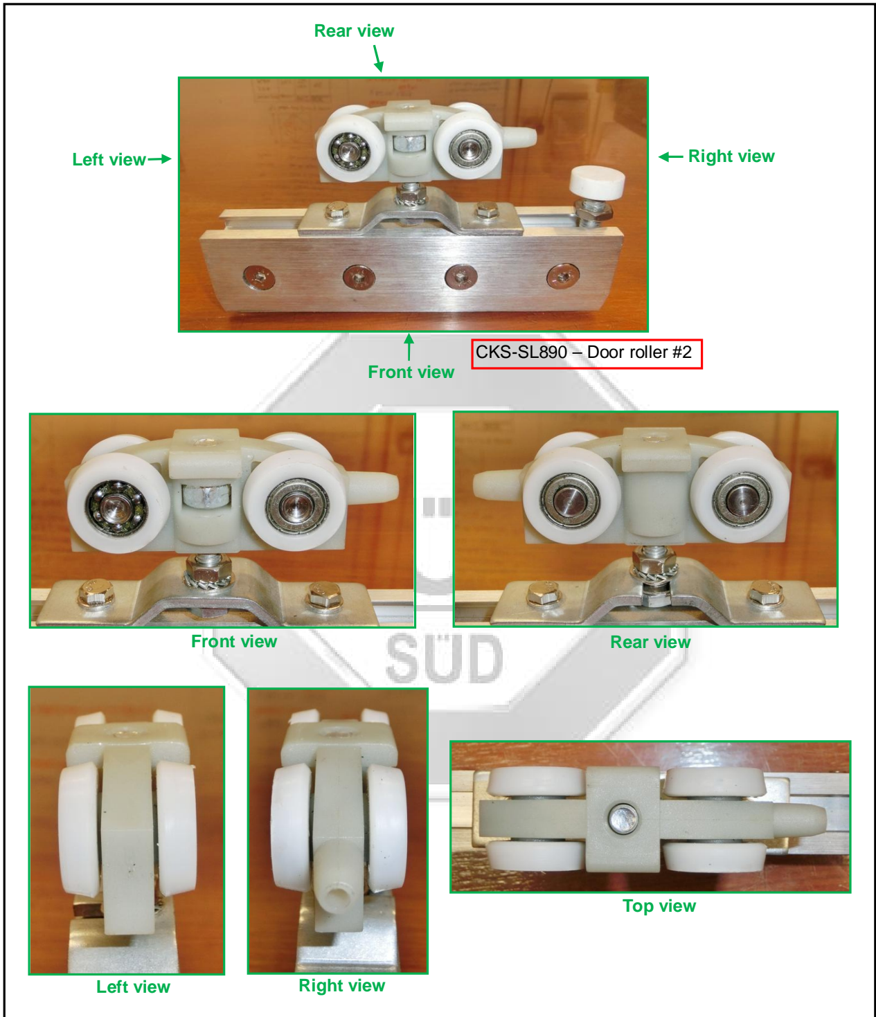
Figure 5: CKS-SL890 door roller after 100,000 cycles of endurance test. (No cracks and wobbling on the wheels was observed after 100,000 cycles of endurance test)
