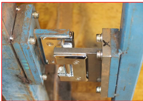
Figure 5: Lower hinge under test (open position)
