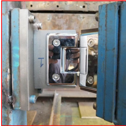
Figure 3: Lower hinge under test (close position)
