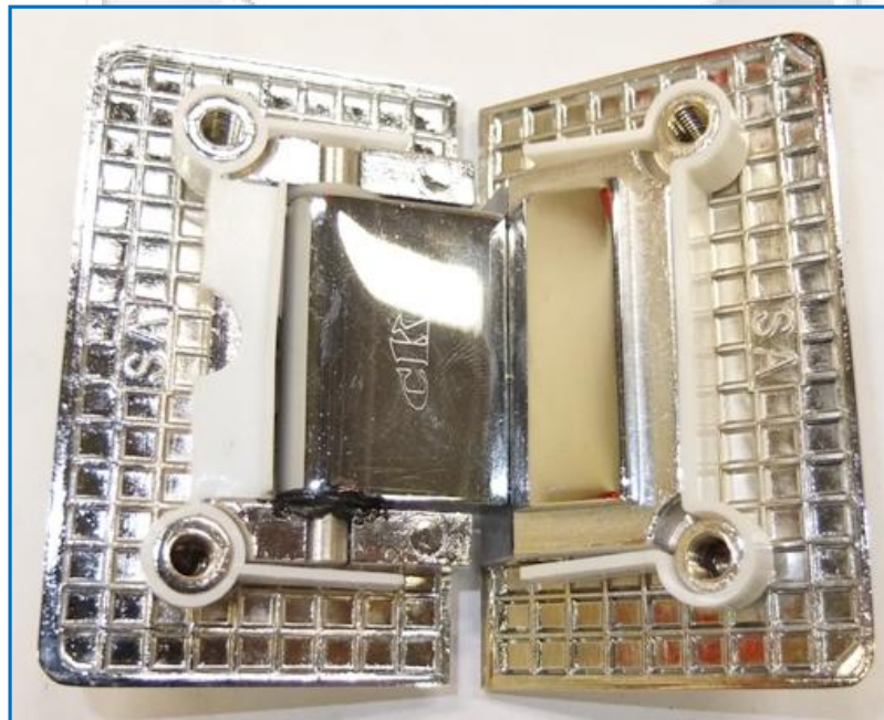
Figure 8: Lower hinge after 60,000 cycles of durability test
