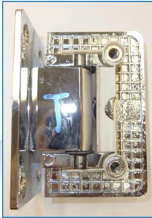
Figure 7: Upper hinge after 60,000 cycles of durability test
