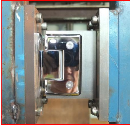
Figure 2: Upper hinge under test (close position)
