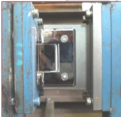
Figure 3: Lower hinge under test (close position)
