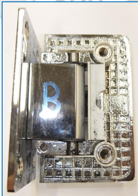
Figure 8: Lower hinge after 60,000 cycles of durability test
