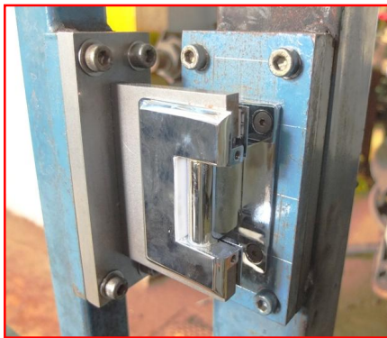
Figure 5: Lower hinge under test (open position)
