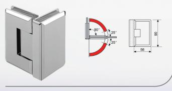
Self return from 25° (either direction) Fit for door thickness: 8, 10mm Door load up to 45kg
