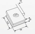
Fit for glass thickness: 10, 12mm Standard cover plate : Stainless Steel
